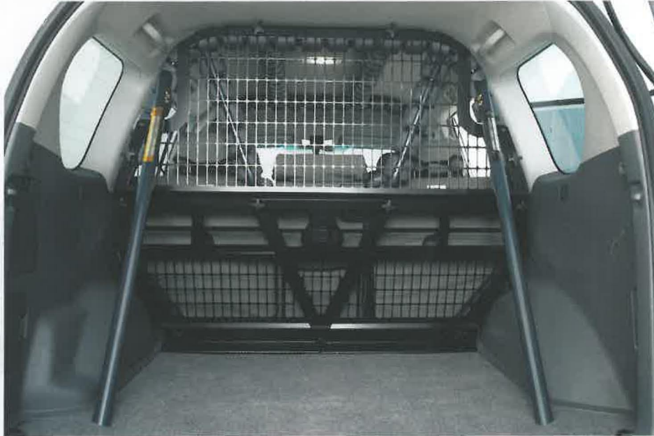
The internal roll over protection system previously obstructed the deployment of side airbags.
